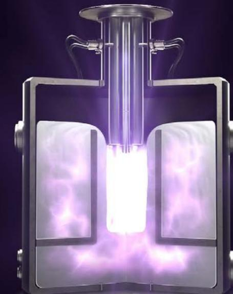
AN ARTIST'S RENDERING OF THE FUSION reaction that takes place within Zap Energy's FuZE-Q reactor. This device uses pulses of electrical current traveling along a central column, which creates a strong magnetic field that confines, compresses and heats plasma to the point of generating fusion.
